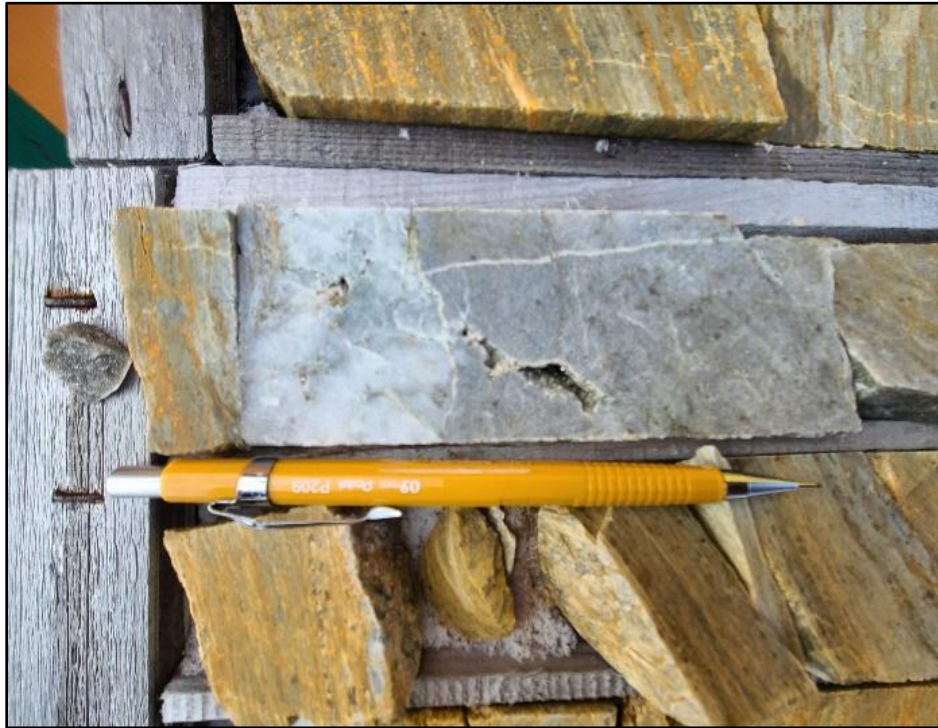
Figure 12-8: Hole HB-11-023 - grey, vuggy silicification and foliated alteration zone lithologies
