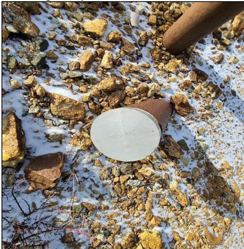
Figure 12-5: Drill hole casing with cap
