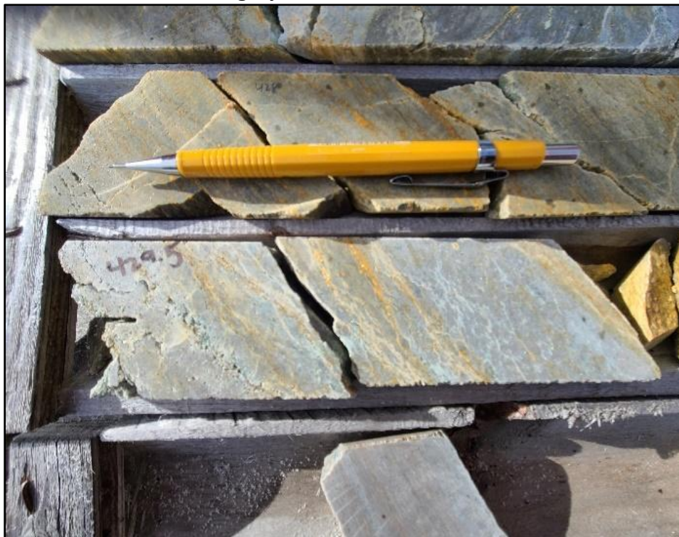
Figure 12-9: Hole HB-11-046 tan to grey silicification and foliated alteration zone lithologies
